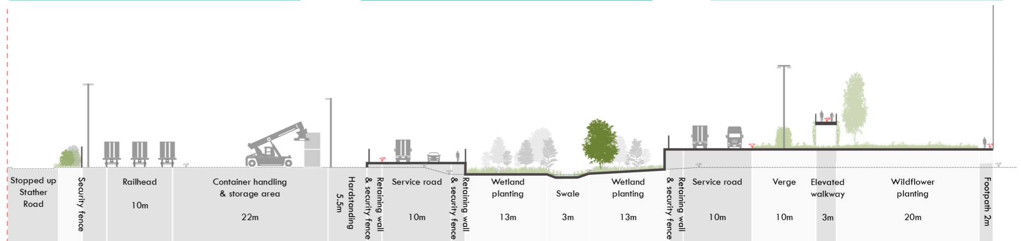
Figure 5.21: Illustrative Railhead and Rail Corridor Sections
